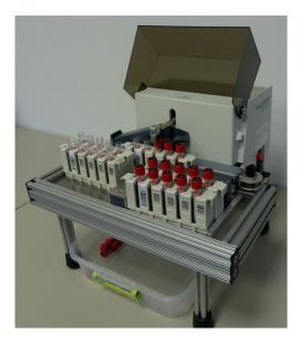
Our Pluggo RHs decapper safely and automatically removes original caps from vacuum sample tubes. Analyzer racks filled with tubes are placed in the inlet channel and are manually forwarded to the decapping station. The device processes one rack at a time. The tubes stay in the racks during decapping. Removed caps are guided to an outlet for collection of biohazard disposal with a detachable chute.
