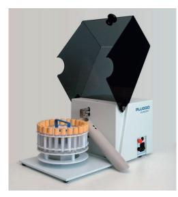
Our PLUGGO Standard decapper is an automated system for the safe removal of original stoppers from vacuum tubes. It processes tubes with pull caps and is a carousel based automated bench-top device that handles all standard vacuum collection tubes.
