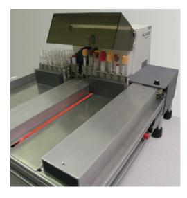
Our Pluggo RH decapper is a compact bench-top device that safely and efficiently removes original caps from blood specimen tubes. Tubes in an analyzer rack are put in the inlet channel; tubes stay in the rack during decapping. The inlet channel holds up to 15 racks that are automatically processed. Racks with tubes that have been decapped are pushed into the outlet channel. Removed caps are guided to an outlet for collection of biohazard disposal with a detachable chute.
